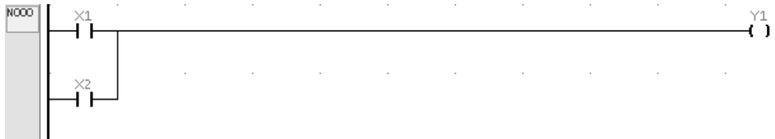
Figure 10.8 Ladder diagram for OR Gate
