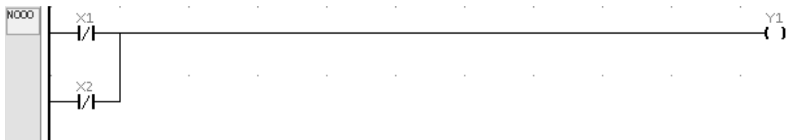
Figure 10.10 Ladder diagram for NAND Gate
