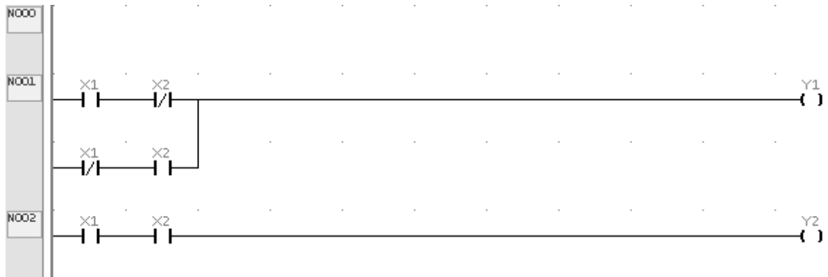
Figure 12.5 Ladder diagram for Half Adder
