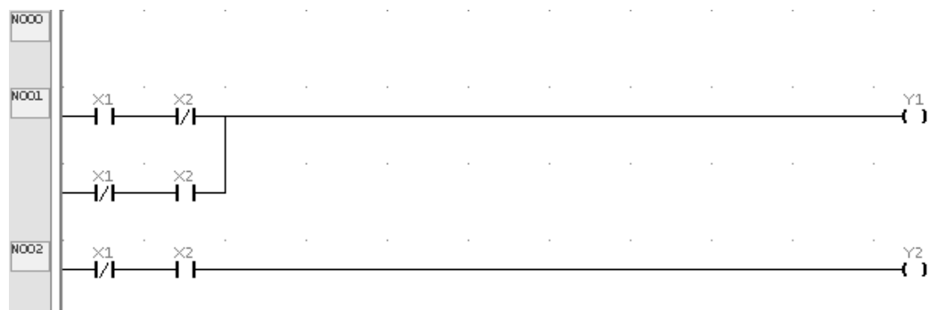
Figure 12.7 Ladder diagram for Half Subtractor
