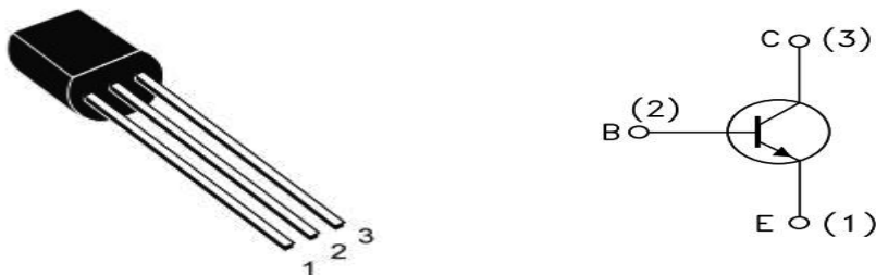
Figure 2: TO-92 package of transistor and its terminals
