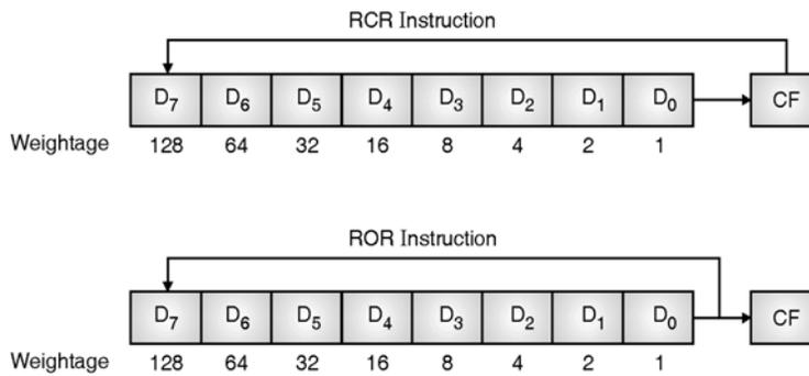
Then D<sub>0</sub> bit goes to the carry flag, hereafter by checking carry flag, number can be tested for odd or even.
