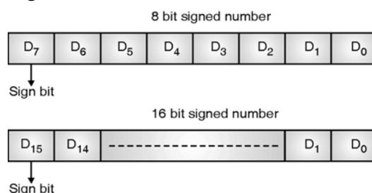
Hence, by checking most significant bit, we can find out a byte or word is positive or negative number. Most significant bit i.e.  $D_7$  or  $D_{15}$  for byte or word can be checked using either ROL or RCL instruction as given in Fig. given below.
