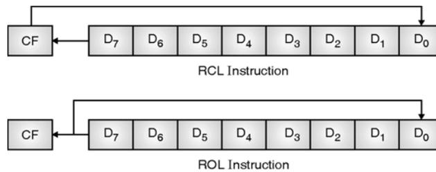
The program for checking odd or even number can be used by replacing **ROR** or **RCR** instruction with **ROL** or **RCL** instruction to check either number is positive or negative.
