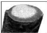
Fig 10: This photograph provided by Dr. C. S. Vishwanath, Bangalore illustrates improper quenching treatment . Note non-uniform hard periphery signifying that the quenching has not taken place all round the periphery. Such bars are produced due to incorrect operation by mill personnel. Such bars should be used only after extensive testing.
