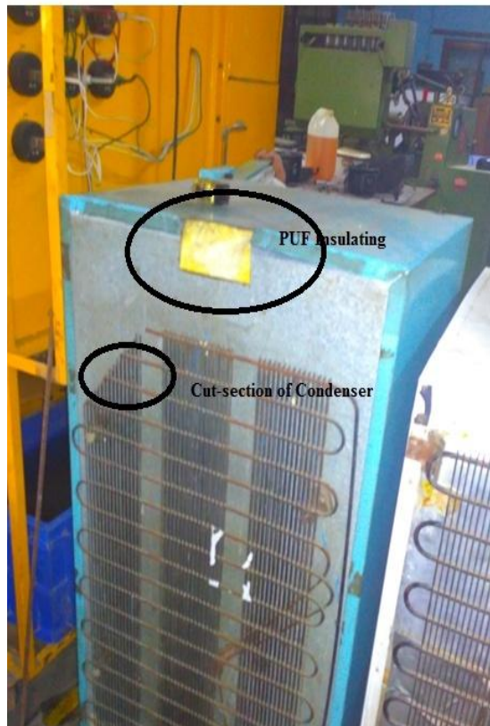
Figure No. 16 Actual Cut-section of household refrigerator representing PUF insulating back panel, condenser coil.
