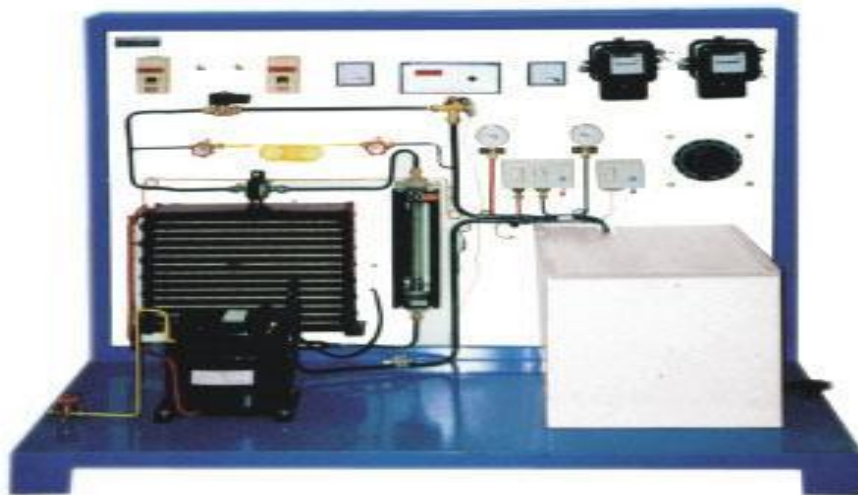
Figure 2 Vapor compression refrigeration Test rig
