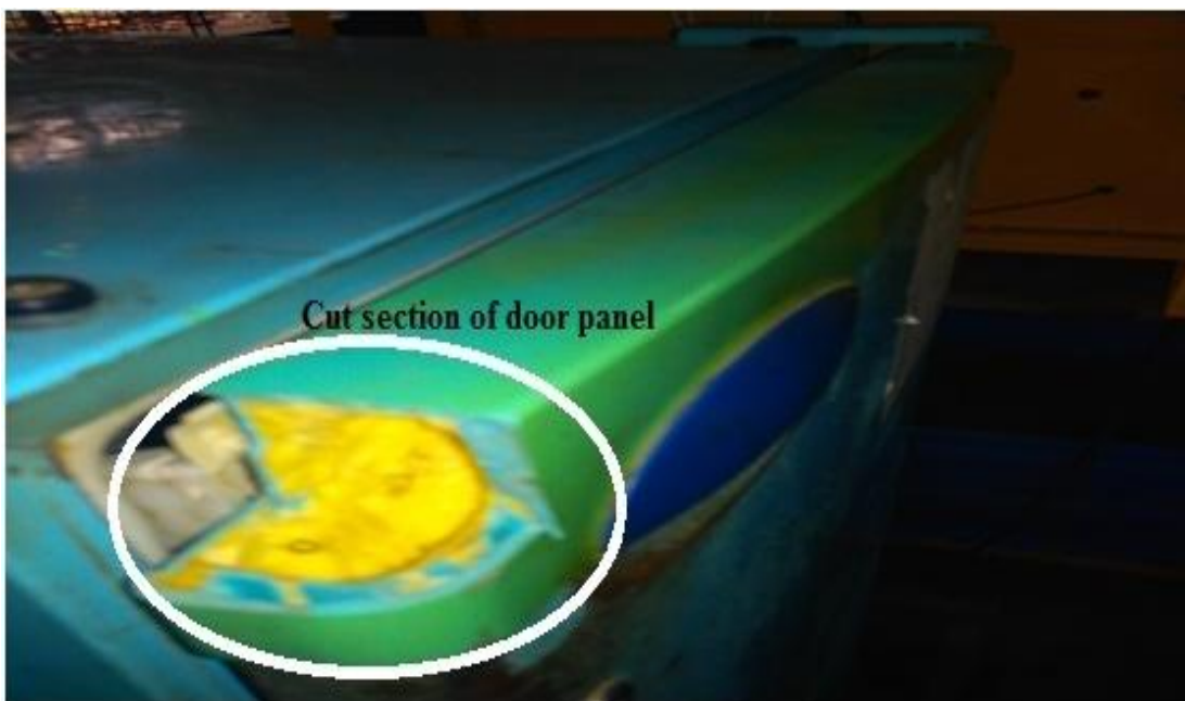
Figure No. 18 Actual Cut-section of household refrigerator representing PUF insulating door panel
