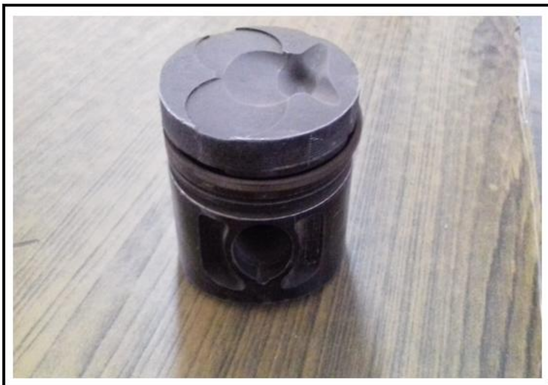
Figure No 6 Pitting of Piston
