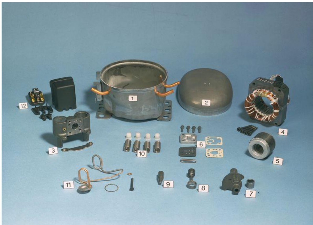
Figure No. 7 Disassembly of Hermetically sealed rotary compressor
