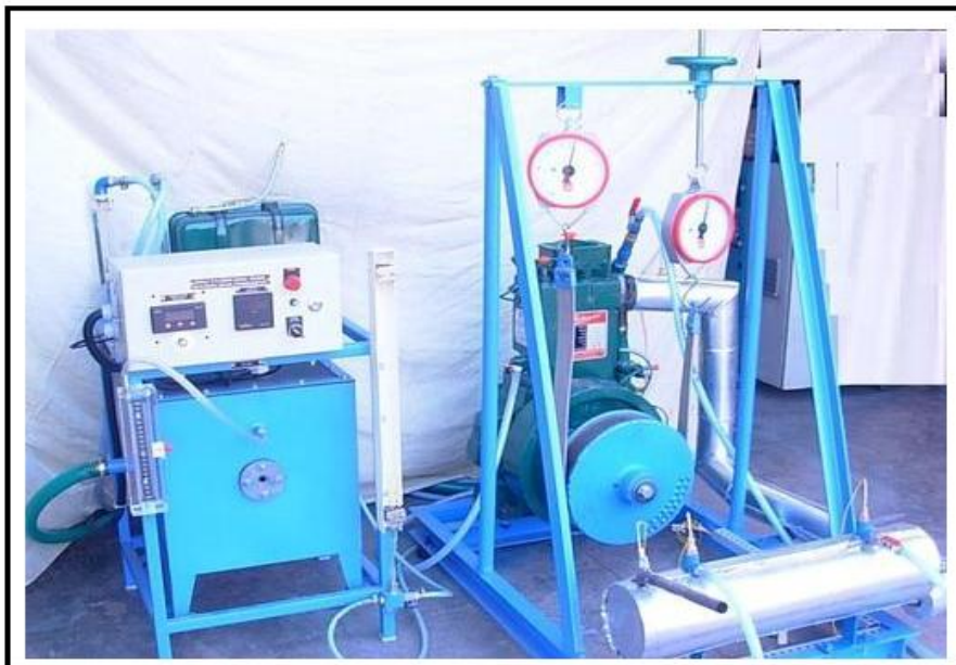
Figure No 2 Diesel Engine Test Rig With Rope Brake Dynamometer
