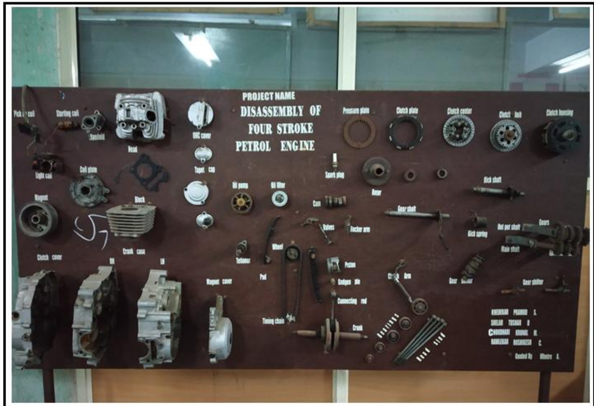
Figure No 5 Dismantling of 4-stroke single cylinder petrol engine
