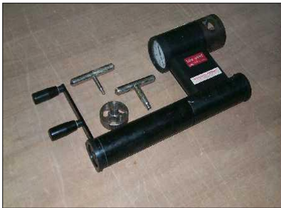
(a) CAPO Test Apparatus with Accessories.
