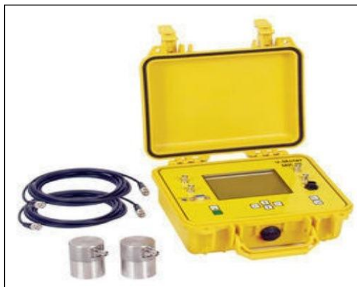
(a) Ultrasonic Pulse Velocity Meter with Probes
