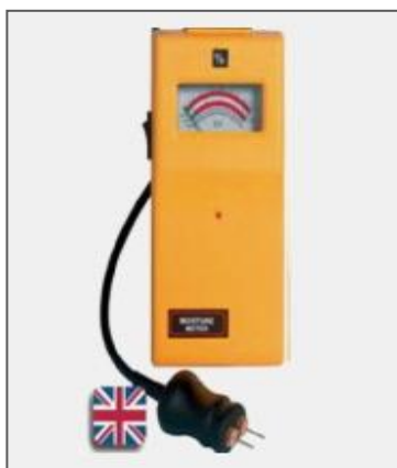
Figure 2: Moisture meter test apparatus
