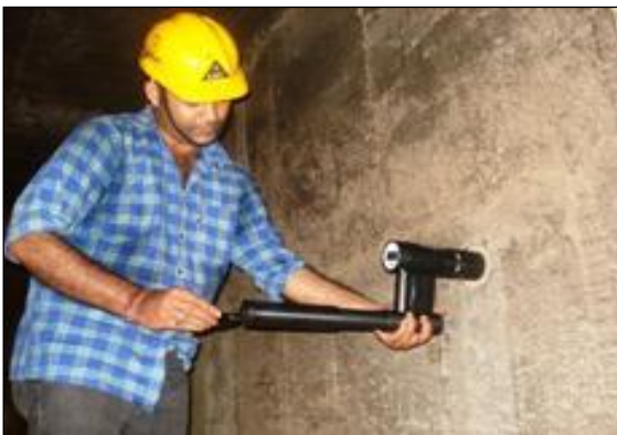
(c) CAPO Test on Column.
