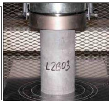
(b) Compression test on core
