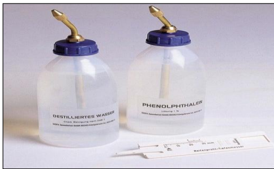
(a) Phenolphthalein solution as indicator.
