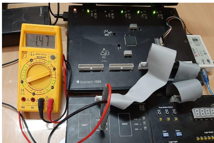
Fig. no. 15.2.a: Lab Practical Setup by set LSB data Bit high Analog output is low voltage
