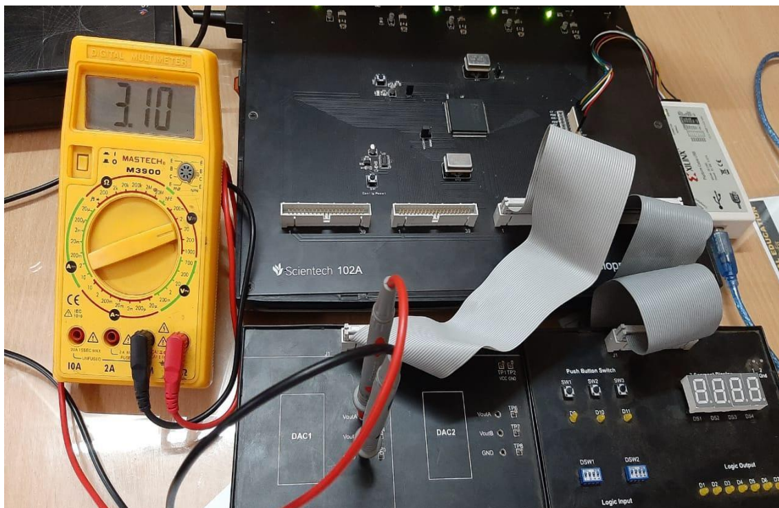
Fig. no. 15.2.b: Lab Practical Setup by set MSB data Bit high Analog output is high voltage
