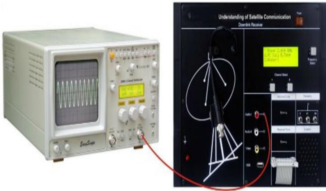
Fig.19.2: Connect Audio-I socket of Downlink Receiver to the Oscilloscope.
