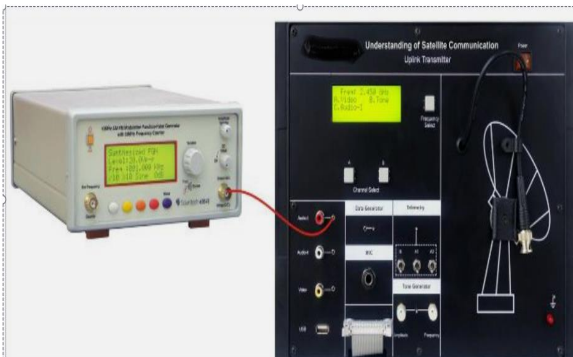
Fig 19.1: Connect Function generator Sine wave output to Audio-I socket
