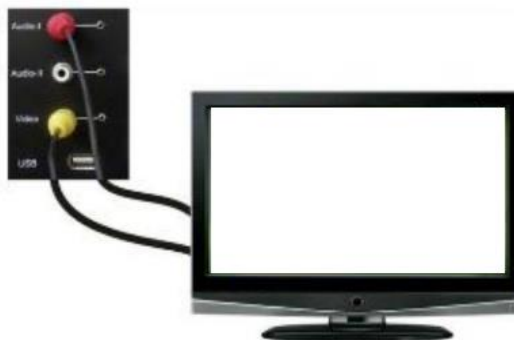
Fig. 16.5: The TV Monitor Connection to Display Video and Audio signal
