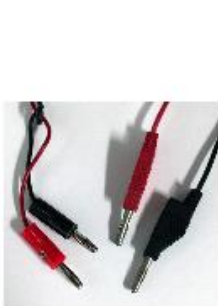
Test leads have banana plugs on one end and pins on the other.
