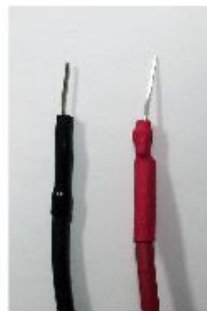
Test leads have banana plugs on one end and pins on the other.
