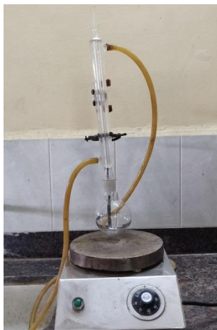
Figure. 1 Reflux apparatus for esterification
