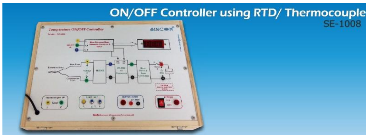
Figure 2: Temperature measurement using ON-OFF controller
