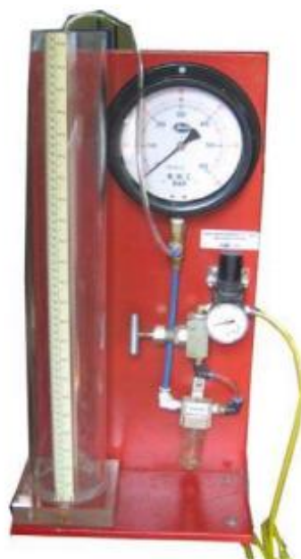
Figure 2: Laboratory Air Purge Liquid Level measurement set up
