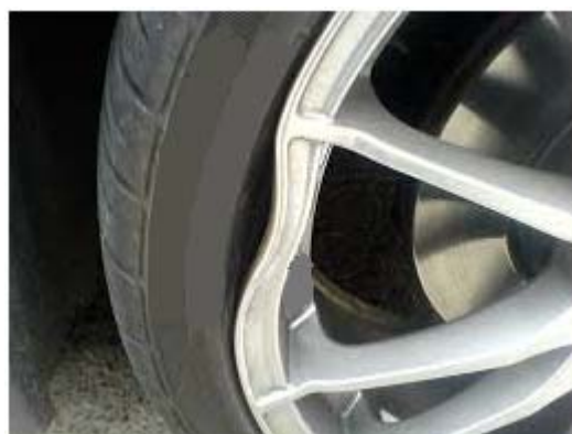
Figure No 12.3: Damaged Wheel rim: a result of rim hitting a pothole and also causes a blown tyre. Replacement of tyre and wheel balancing is not sufficient as a slight shimmy is experienced by the driver and vehicle occupants.
