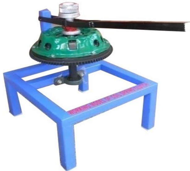
Figure 2.2: Working Model of Single Plate Clutch
