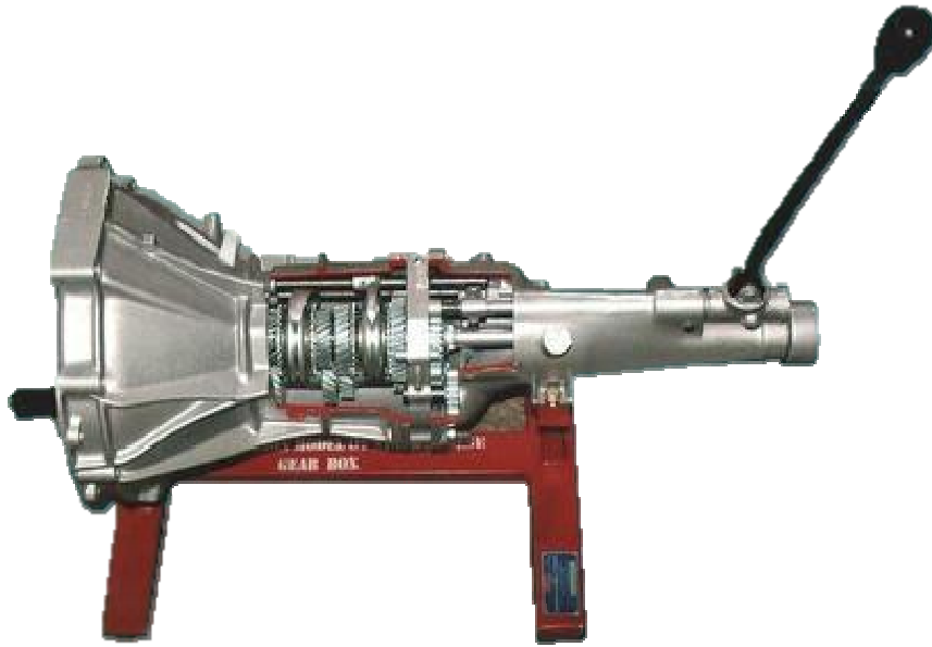
Figure 5.4: Working Model of Synchromesh Gear box
