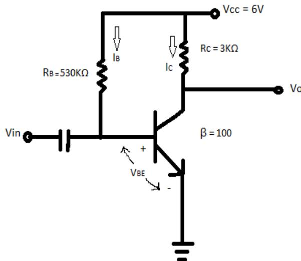
Also draw the DC load line and determine the operating point.
