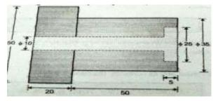
13. Prepare operation process sheet and sequence of operation for the ring nut assume suitable cutting parameter and raw material 50×10mm blank of carbon steel.
