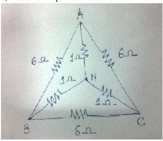
9) Find loop current and current flowing through  $1\Omega$  using mesh analysis.
