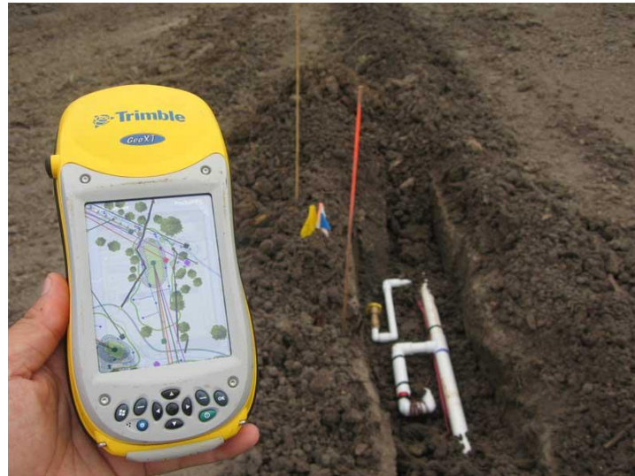
Fig. 3.4: Handy GPS Device used to Map an Area
