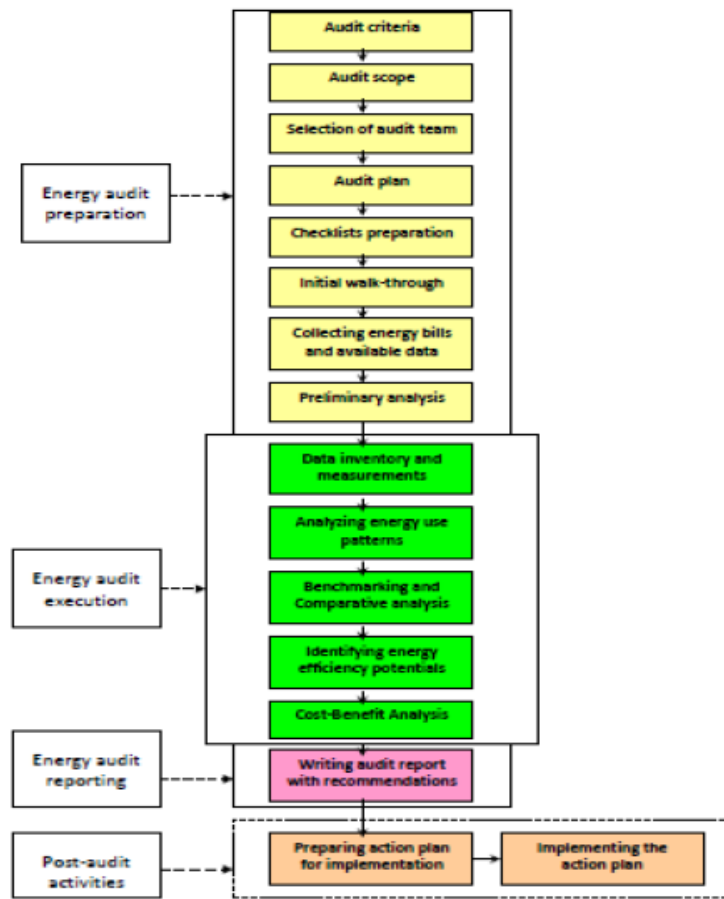
Fig. 4.3: Detailed Energy Audit Process (Source- Hassan et al)
