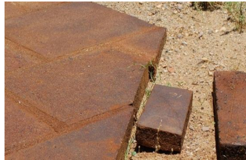
Fig. 2.34: Ferrock as blocks
