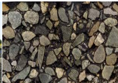
Fig. 2.16: Stone Mastic Asphalt
