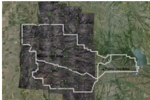
Fig. 3.9: Green Dots showing GCP's
