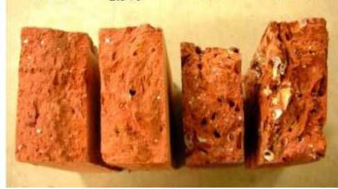
Fig. 2.4: C/S Of Bricks With Varying Percentage of Cigarette Butts
