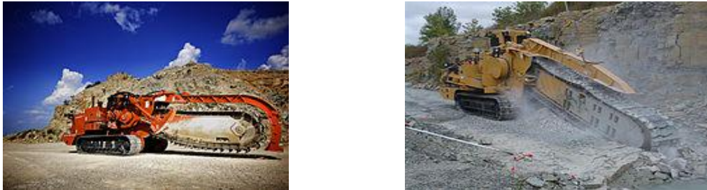
Fig. 3.17: Chain Trencher with Digging Chain
