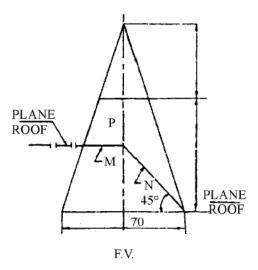
3 A cone of base diameter 60 mm and 70 mm long axis rests on HP on its base. It is cut by a section plane perpendicular to VP and inclined 45° to HP passing from a point on axis 35 mm from apex. Draw development of lateral surface of cone.
